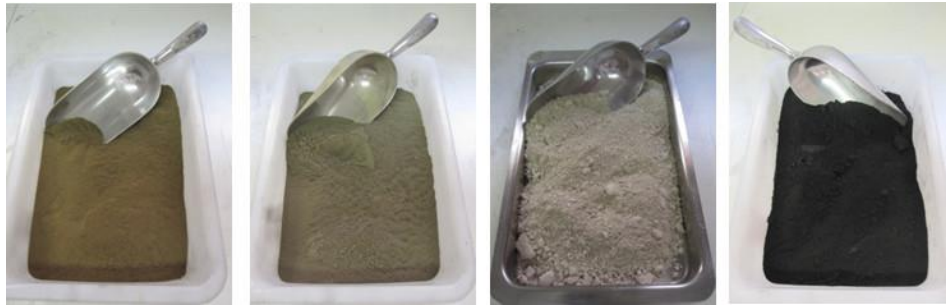
Figure 1. Mineral additives used (left to right): sewage sludge ash (SSA); fly ash (FA); marble dust (MD); rice husk ash (RHA).
