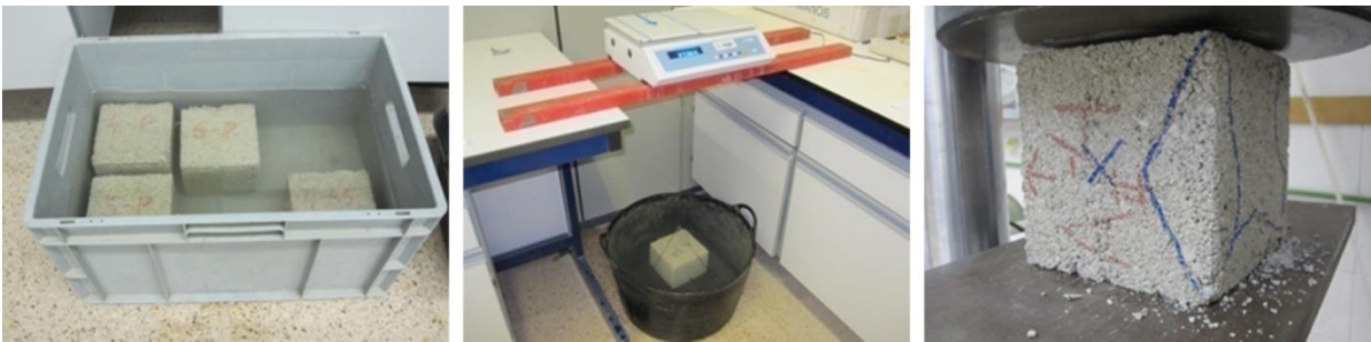
Figure 3. Concrete specimens tests procedure (left to right): Specimens submerged to saturation; density and absorption; compressive strength.
