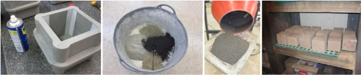
Figure 2. Concrete specimens fabrication procedure (from left to right): cubic specimens 150 mm sides; premixing of dry components; mixing of concrete; preservation of the specimens in controlled humidity chamber.
