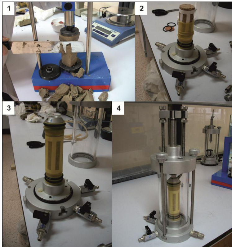
Fig. 2. Screenshots of a geotechnical test (e.g. CD triaxial test) included in the virtual laboratory tests library (Tomás et al., 2013c).
