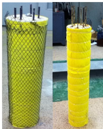
Figure 1. Anodic system composed by a Ti-RuO 2 mesh embedded between two absorbent polymeric layers, wrapping concrete specimen.
