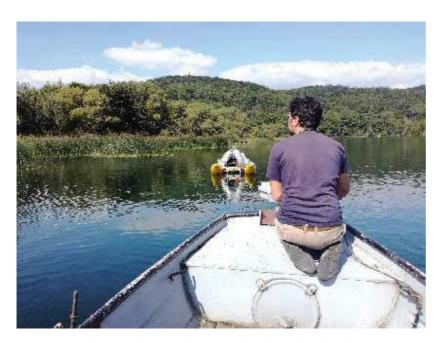
Team member Zakaria Ghazoui checks a hydrophone unit suspended beneath a raft in Laacher See. Credit: Corentin Caudron
