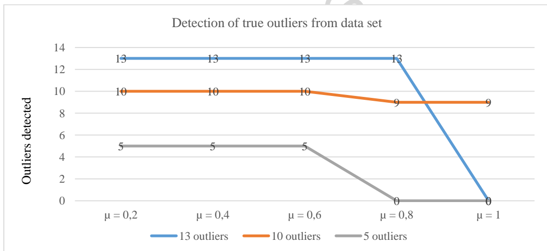
Figure 11. Number of real outliers detected in the data set as a function of the number of artificial outliers introduced and the threshold \mu .
