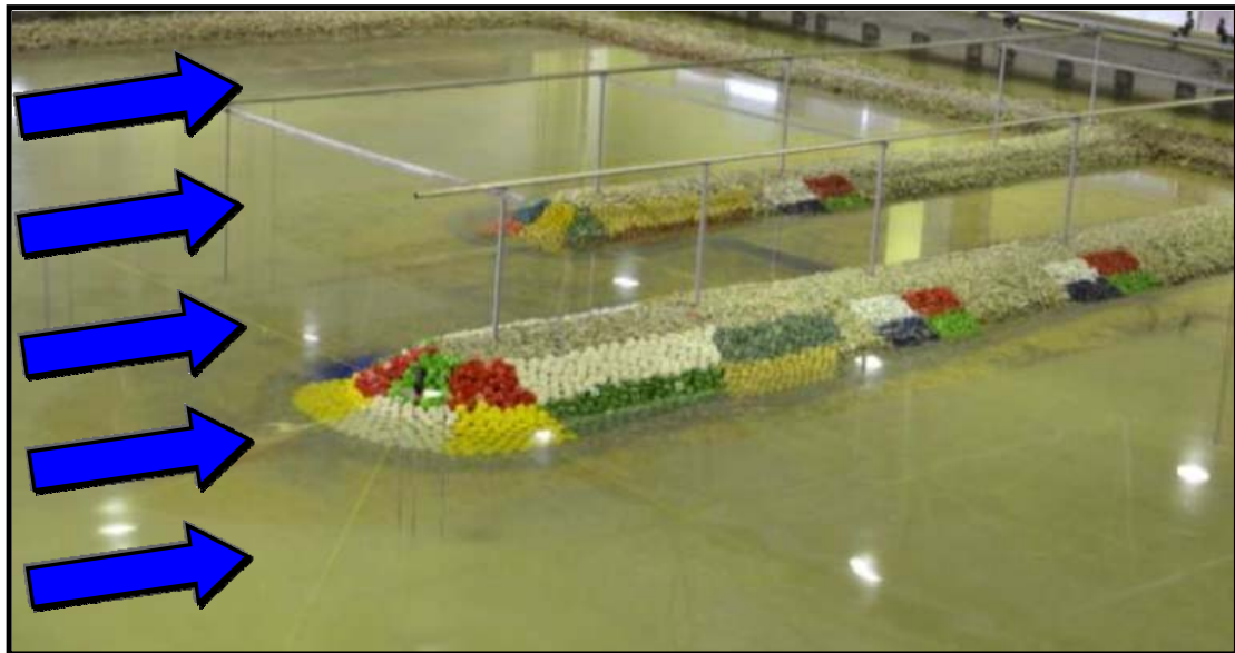
Figure 5. 3D CITEEC wave basin and 1/45-scale model with double-layer 5-tonne quarrystone and single-layer 12.1-tonne and 23.2-tonne Cubipod armors.
