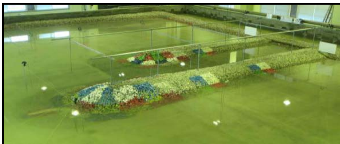
Figure 3. 3D wave basin and 1/45-scale model with double-layer 5-tonne quarrystone and double-layer 20-tonne and 35-tonne cube armors.
