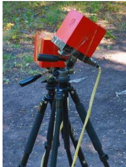
Fig. 11. Picture of both magnetic field sensors spatial arrangement in shielding space point for closed loop control by system of active shielding model
