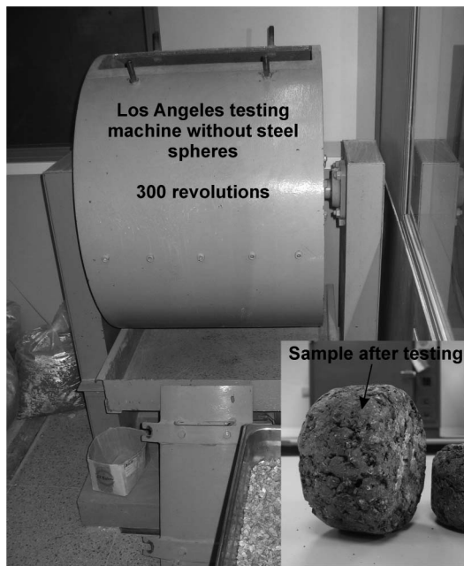
F3:1 Fig. 3. Cantabro test machine and bituminous mix after testing
