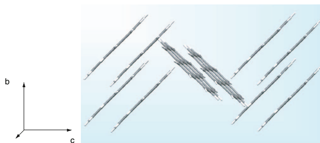
FIG. 7. Unit cell of the coronene crystal structure viewed along the crystallographic b axis.
