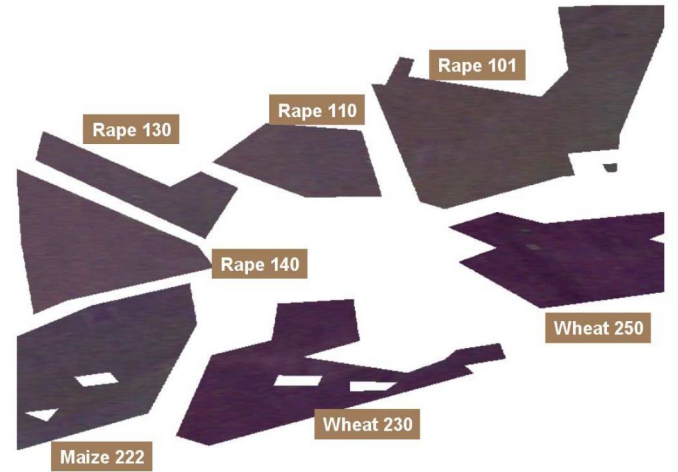
Fig. 4. RGB image of the Agrisar 2006 test site. R = HH, G = HV, B = VV.
