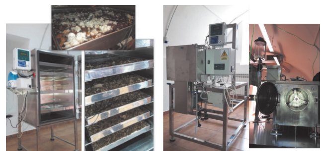
Fig. 3. a) Tray bioreactor, b) Horizontal bioreactor with mechanical mixing
