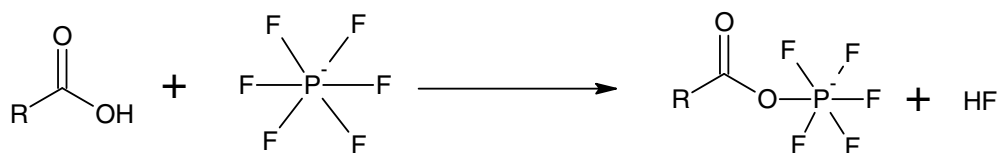
Figure 5. Proposed reaction for the interaction between the \text{PF}_6^- anion of the ionic liquid and the surface carboxylic groups.
