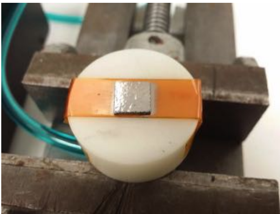
Figure 4.3: A HOPG sample secured to the chuck via vacuum seal [57].
