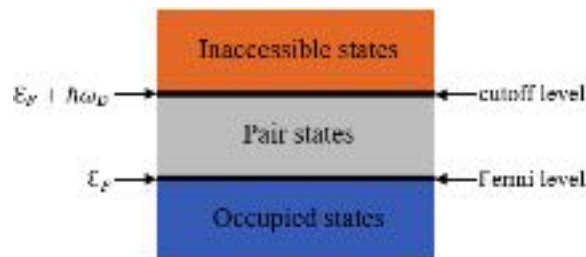
Figure 2.8: Pair states accessible to delocalization of a Cooper pair.
