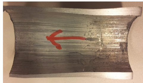
Fig. 6. Longitudinal section of stretched abrupt transition manufactured without releasing pressure from billet for mandrel drawback, (ED ←)
