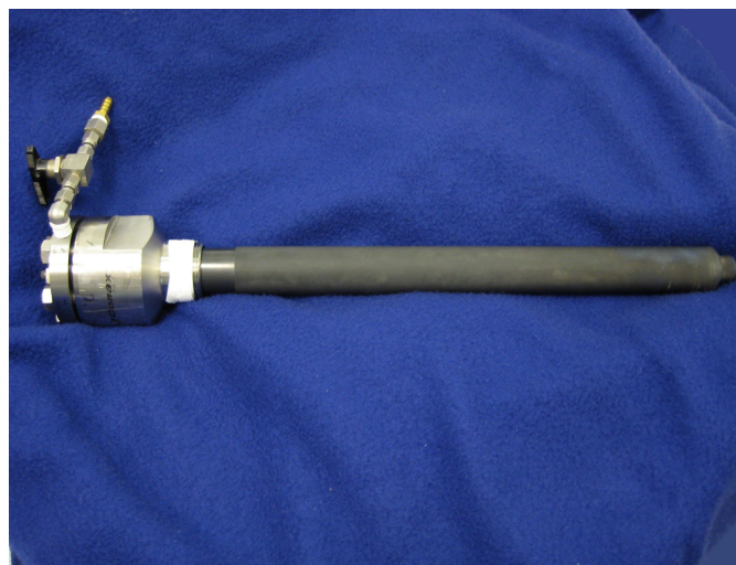
Fig.1. The novel all-SiC probe assembly with sealed pressure connector with optical window.
