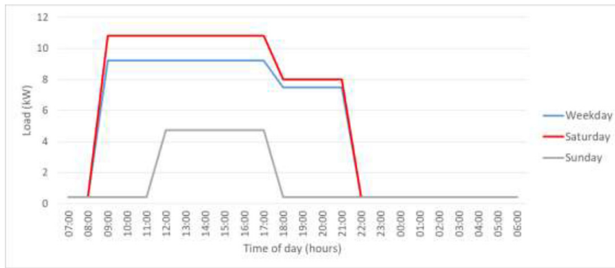
Fig. 1. Olowos plaza hourly load demand for a typical weekday, Saturday and Sunday.
