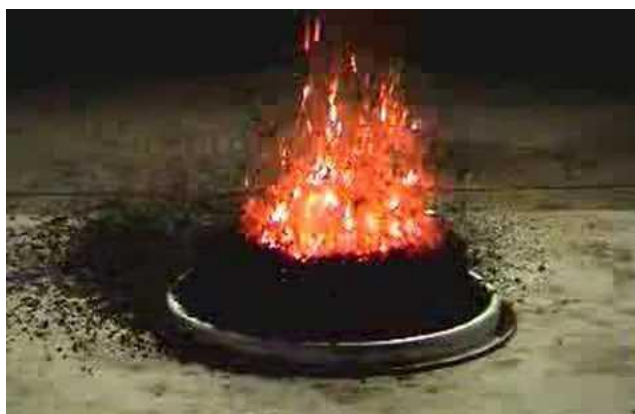
Fig. 1. Ammonium dichromate volcano reaction.
