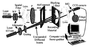
Figure 1 Experimental set-up 1 for zero spatial frequency recording
