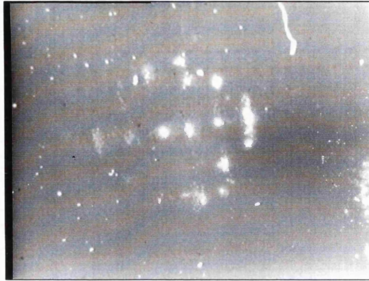
Figure 2.49 Photomicrograph of unpolished face of the \text{LiNbO}_3 crystal showing pattern of damage.
