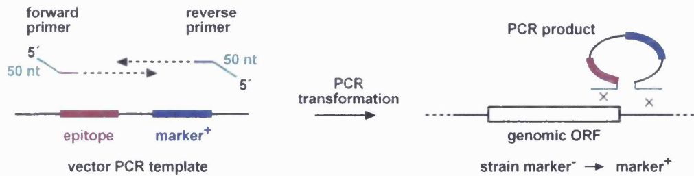
Figure 7.1. Schematic overview of PCR-based epitope tagging of genes by homologous recombination.
