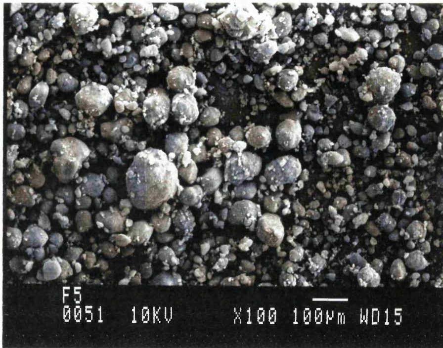
Fig. 4.1.9. FCC with 5% CAB-O-SIL ( \times 100 ).
