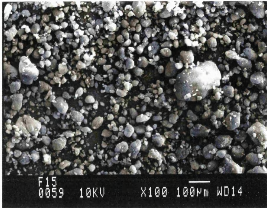
Fig. 4.1.13. FCC with 15% CAB-O-SIL ( \times 100 ).
