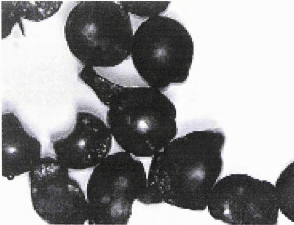
Figure 6.6. Electron microscope photographs of steel particles ( \rho = 7510 \text{ kg/m}^3 , d_p = 110 \text{ }\mu\text{m} ).
