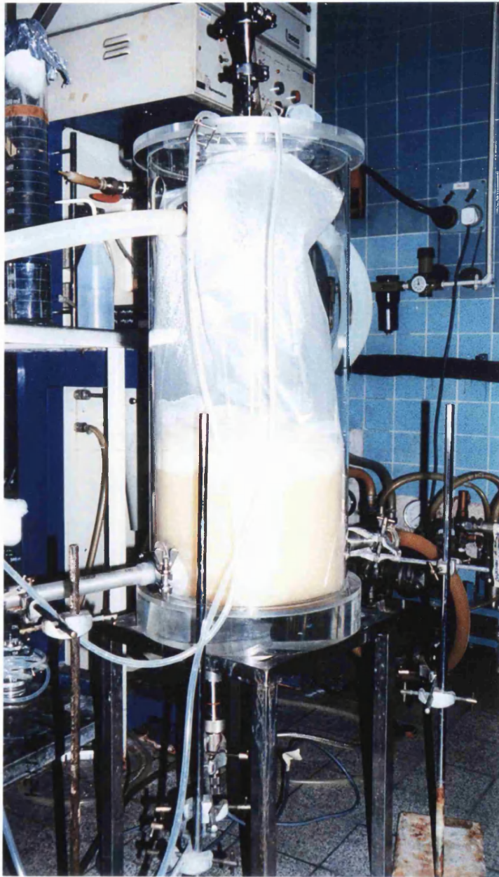
Figure 24 – 14 L plunging jet bioreactor in operation with a microbial fermentation
