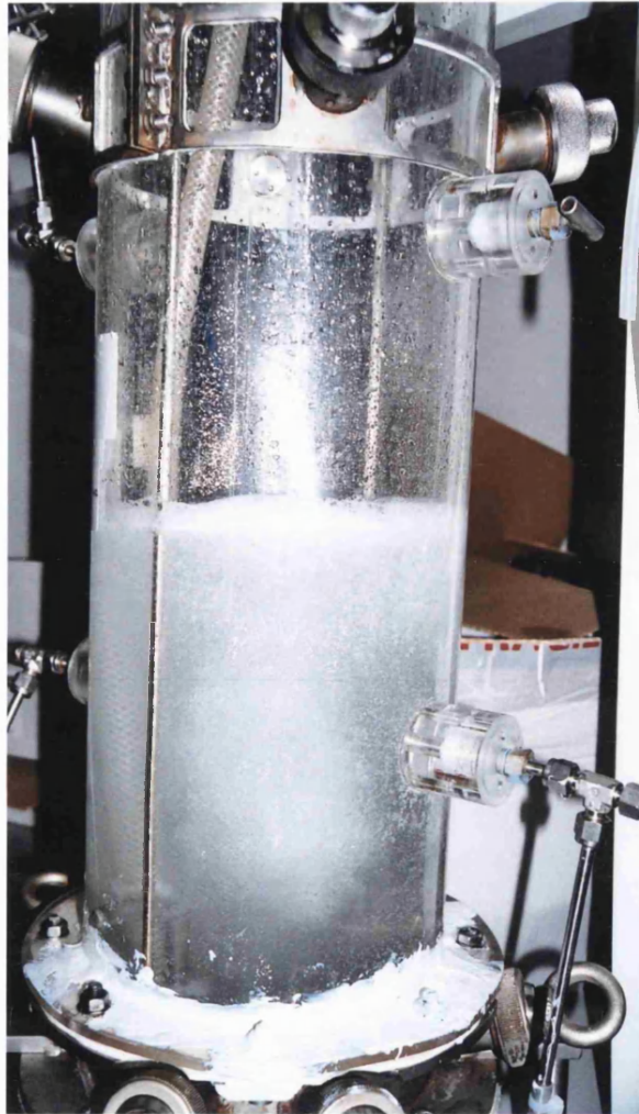
Figure 46 B – Picture of the plunging jet reactor with the ‘foam effect’
