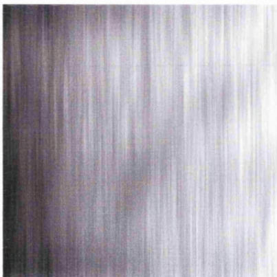
2.14 vi Inverse transform of above. The horizontal line of the FFT represents this pattern of vertical lines with a luminance gradient. This represents the luminance gradient within the original 'blank screen' image.
