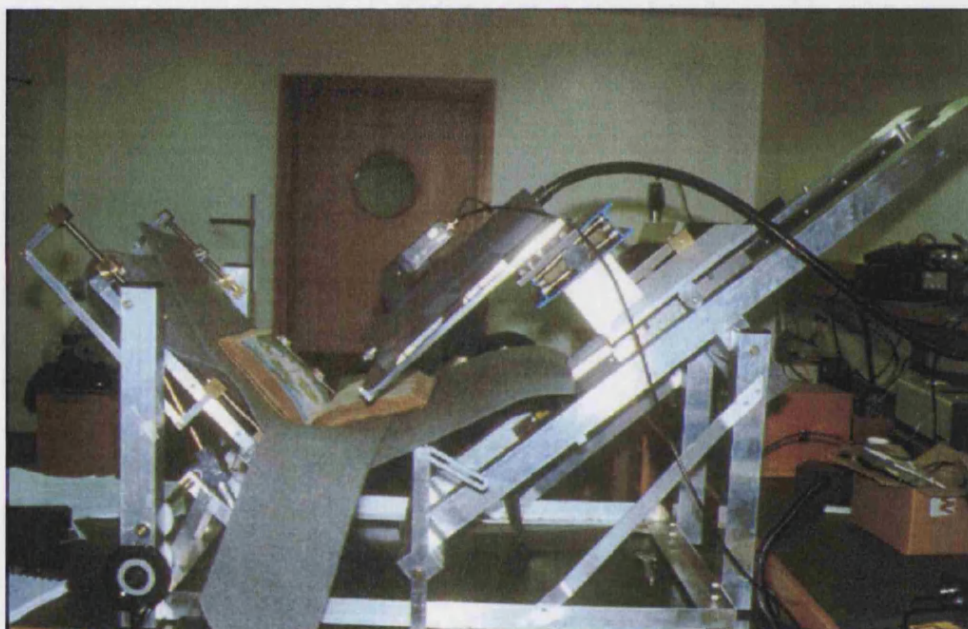
Figure 2.9: The book cradle and remote probe assembly.
