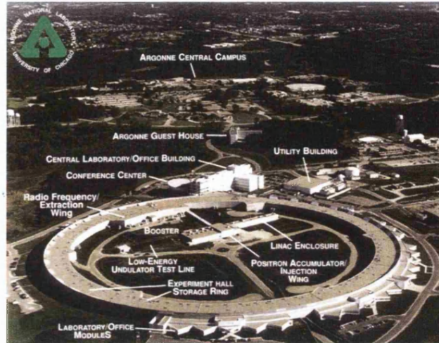
Figure 2-4 Picture of the Advanced Photon Source (APS), a third generation synchrotron located at the Argonne National Laboratory (ANL) south of Chicago (Illinois, USA).
