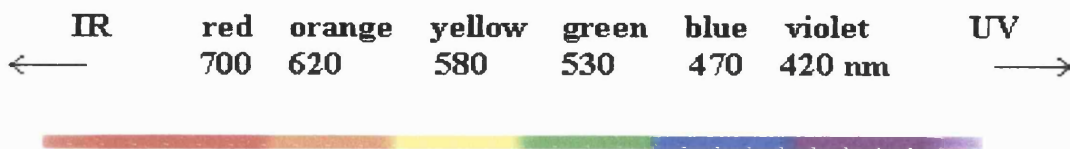
Figure 1.5 The visible region of the electromagnetic spectrum. 20
