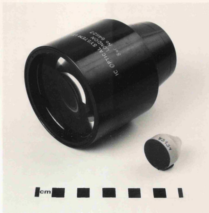
Fig 2.8. The MIC fibre taper and the CCD-IPCS coupling lens
