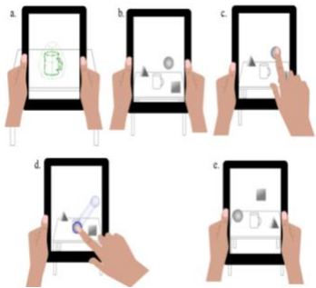
Figure 4: Performing a trial with the easy interface beginning with a. Target object scan; b. AR objects view; c. Object selection; d. Dragging the AR objects to target object; e. AR objects rearrange and tasks b – d are repeated.
