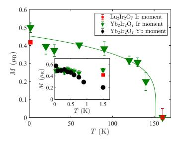
FIG. 6. Temperature dependence of the refined magnetic moment on Ir in  $Lu_2Ir_2O_7$  and  $Yb_2Ir_2O_7$ , assuming only AIAO order. The line is to guide the eye. (Insert) Low-temperature region showing also the moment on the Yb sublattice assuming only a ferromagnetic component. Data below 1 K were measured in a dilution fridge.
