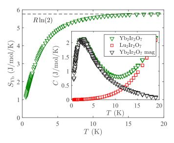
FIG. 8. Heat capacity and entropy per mole of Yb for our  $Yb_2Ir_2O_7$  sample.
