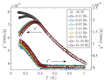
FIG. 7. The real ( $\chi'$ ) and imaginary ( $\chi''$ ) parts of the measured ac susceptibility signal from Yb<sub>2</sub>Ir<sub>2</sub>O<sub>7</sub>, showing that spin freezing sets in at  $T \simeq 0.4$  K.
