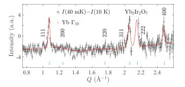
FIG. 10.  $I_{\text{mag}}^{40 \text{ mK}}$ (Yb) calculated using Eq. (B1), along with a refinement of the Yb magnetic structure.
