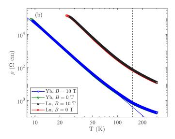
FIG. 9. Resistivity of Lu<sub>2</sub>Ir<sub>2</sub>O<sub>7</sub> and Yb<sub>2</sub>Ir<sub>2</sub>O<sub>7</sub> in zero field and in an applied field of 10 T. The dashed line indicates the magnetic ordering temperature from the magnetization measurements. Below  $\sim$ 25 K, the resistivity of the Lu<sub>2</sub>Ir<sub>2</sub>O<sub>7</sub> sample is higher than the instrument limit.
