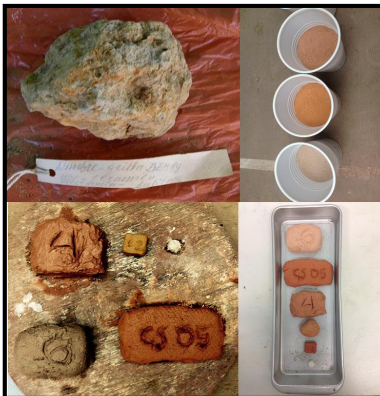
Figure 6-3. Clay samples obtained at Museo Ceccarelli and during fieldwork 2017 with Aura. Inset (top left to right): Clay sample from Galito-Upper Rio Negro; Ground clay samples from Aura's excursion -Black, Yellow and Red clay respectively-; Wet briquettes before firing (left to right: 4,2,1,6,5); Dry briquettes after firing (Top to bottom: 6,5,4,3,2,1). Source: N. Lozada 2017.
