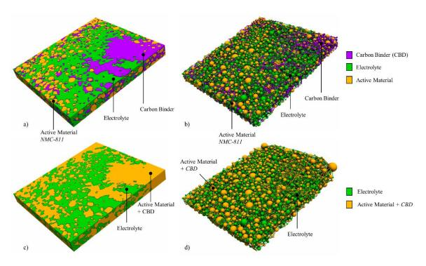
Figure 2 a) X- $\mu$ CT image of lithium nickel manganese cobalt oxide (LiNi<sub>0.8</sub>Mn<sub>0.1</sub>Co<sub>0.1</sub>O<sub>2</sub>) cathode, b) Extracted three phase network of (a), c) Two phase image of porous cathode where active material and CBD correspond to one solid phase, d) Extracted two phase network of (c)
