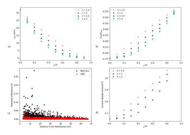
Figure 8 a)Effective electronic conductivity of solid matrix (NMC+CBD) vs nanoporosity of CBD, b) Effective diffusivity of Li-Ion in electrolyte phase vs nanoporosity of CBD, c) Potential difference in solid matrix vs distance from membrane at  $\varepsilon_{CB}=0$  and n=3, d) Current density of solid matrix vs CBD nanoporosity.
