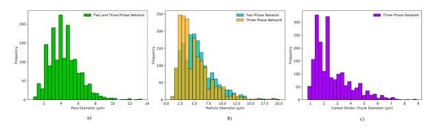
Figure 3 a) Pore size distribution of electrolyte phase in both two and three phase network, b) Active material particle size distribution in two and three phase network, c) Carbon binder particle size diameter in three phase network
