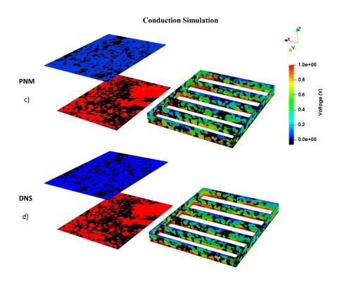
Figure 6 (a) and (b) Comparison of DNS and PNM model in pure diffusion simulation, (c) and (d) DNS and PNM model comparison in pure conduction simulation
