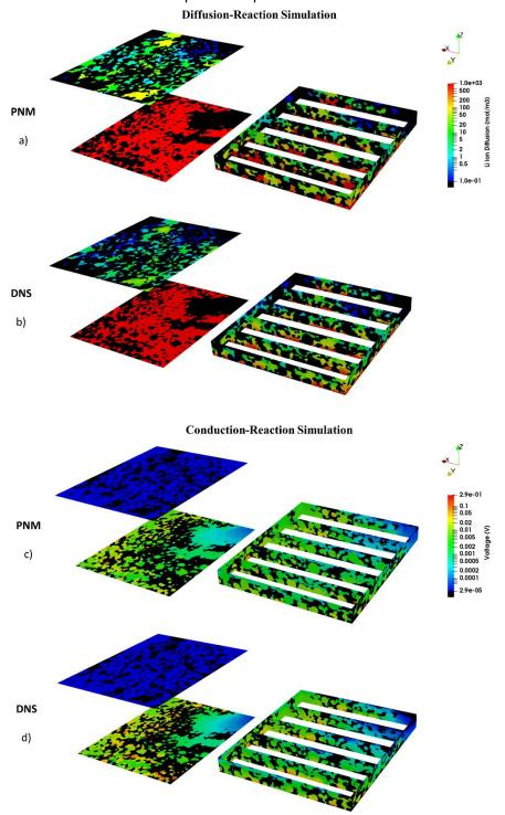
Figure 7 a) Direct Numerical simulation of Li ion diffusion and reaction, b) Pore network modelling simulation for same case as in (a), c) Direct numerical simulation of conduction-reaction in active material and carbon binder phase, d) Pore network modelling simulation of same case as (c)
