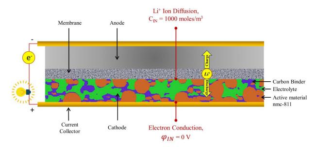
Figure 4 Schematic diagram of full cell lithium Ion battery. The applied boundary conditions are shown in red color.
