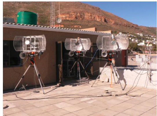
Fig.3- Antennas on pedestals at the location of the monostatic transceiver radar node
