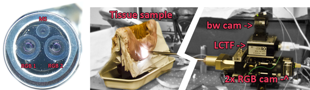
Figure 3.4: Left: The front of the laparoscope and the three camera multiplex; Right the experimental configuration: the scope is positioned perpendicular to the tissue surface as mounted on a translation stage. The axis of motion of the translation stage is normal to the view direction.
