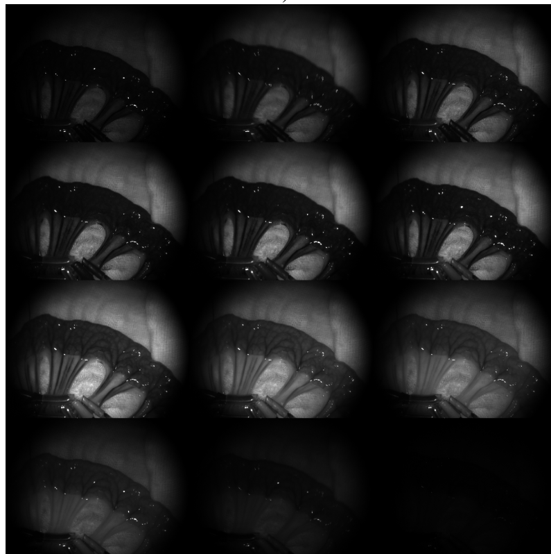
Figure 4.3: a) In vivo experimental configuration for imaging a section of porcine bowel, overlaid is a reconstructed synthetic RGB image (from captured MSI stack and RGB response) with illustrative heat map of THb concentrations. b) A sample MS stack captured by the device imaging at 490nm to 710nm at 20nm increments, from left to right top to bottom. Full capture stack includes 10nm increments and ranges from 450nm to 720nm.
