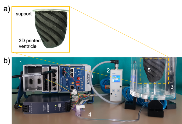
Figure 7. 3D printed model of D_4 (a) and experimental setup in configuration for D_4 (b) with indication for the control unit (1), electrovalve (2), pressurization chamber (3), pressure sensor (4) and 3D printed ventricle (5).
