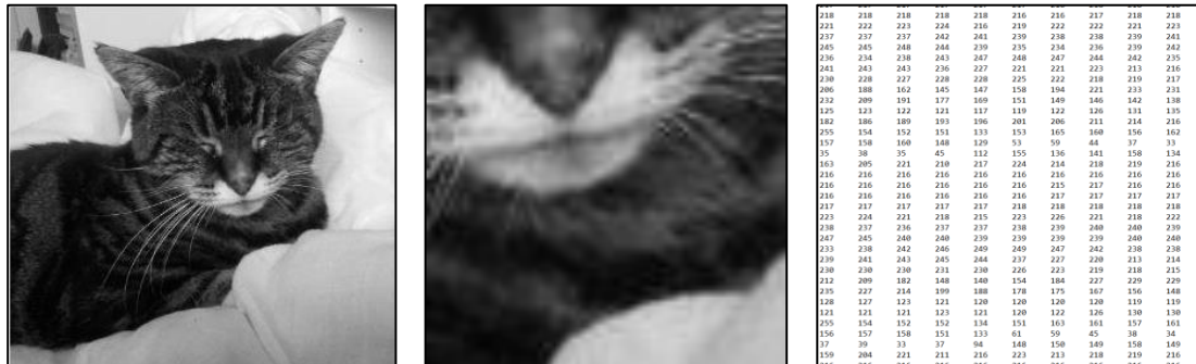
Figure 4.3: Digital images are actually arrays of numerical values. (A) Depicts a grayscale image. (B) Depicts a magnified detail (showing the pixels), and (C) Depicts a magnified detail of the numerical values of those pixels
