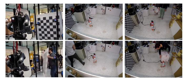
Fig. 2. Illustration of conducted experiments - Left: WALK-MAN v2.0 and VO outliers, Middle: NAO and VO outliers, Right: NAO and LO outliers.
