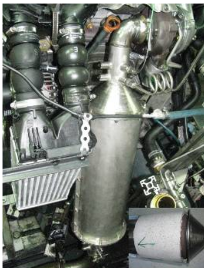
Figure 2. Picture of the DPF holder fitted to the diesel engine exit.
