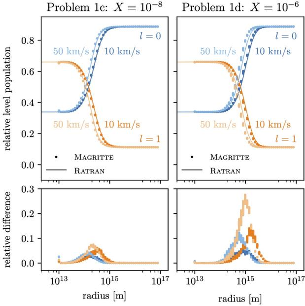
**Figure A1.** Comparison of the results for Problem 1 c/d, obtained with MAGRITTE (dots) and RATRAN (lines) both on a model mesh with 50 shells. The indicated velocities are the  $v_{\infty}$  for each model. The relative difference of two values is measured as twice the absolute difference over their sum.
