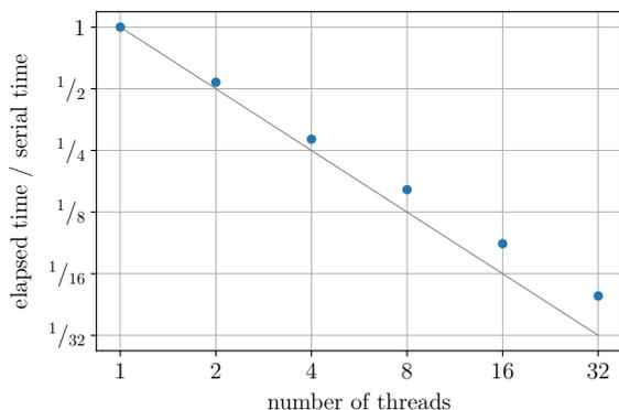
**Figure 11.** Plot of the (strong) scaling of MAGRITTE’s parallelisation for shared-memory systems. The dots indicate the relative timings and the grey line indicates the ideal scaling behaviour. Timings are averages over seven runs performed on one 32-core Intel Skylake node of the CSD3 cluster. (Hyper-threading was disabled for these runs such that the number of threads effectively corresponds to the number of cores used.)
