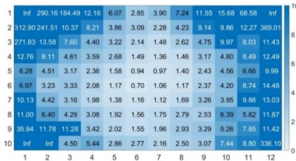
Fig. 5. Pre-Minimiser heatmap of the median localisation error across the arena. Each cell represents a 40 cm × 40 cm region in the arena.
