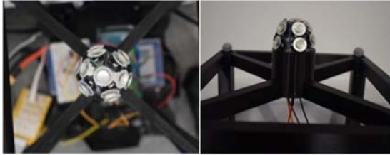
Fig. 1. 'Omnidirectional' US transducer array for the emitter.
