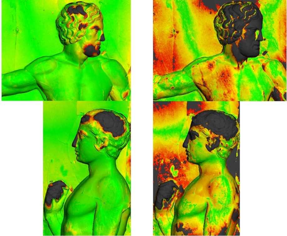
Figure 1. Deviation maps on the left show figures 5 (above) and 6 (below) of West Frieze III at 5 mm maximum deviation: greyscale > 5 mm deviation; red > 3 mm deviation; yellow > 1.5 mm deviation; green < 1.5 mm deviation. Images on the right show the same figures at 1 mm maximum deviation: greyscale > 1 mm; red > 0.6 mm; yellow > 0.3 mm; green < 0.3 mm. Data applied to Elgin cast.
