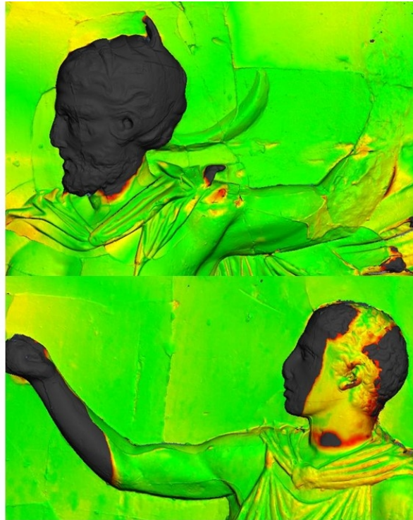
Figure 3. Deviation maps of figure 15 (above – West Frieze VIII) and figure 23 (below – West Frieze XII) at 5 mm maximum deviation: greyscale > 5 mm deviation; red > 3 mm deviation; yellow > 1.5 mm deviation; green < 1.5 mm deviation. Data applied to Elgin casts.
