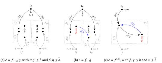
Fig. 6. Schematic depiction of the Thompson construction for guarded union, sequencing and guarded loop operators. The initial psuedostates of the automata for f and g are depicted in gray. Transitions in red are present in the automata for f and g, but overridden by a uniform extension with the transitions in blue.
