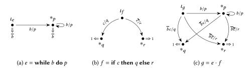
Fig. 7. Concrete construction of an automaton using the Thompson construction. First, we construct an automaton for e, then an automaton for f, and finally we combine these into an automaton for g. In these examples, p, q, r are single action letters, not arbitrary expressions.
