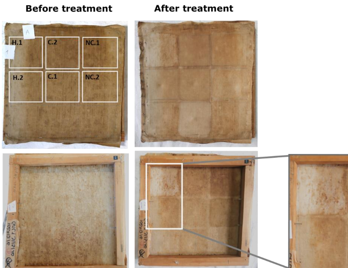
Figure 7.14: Linen lining canvas treated with the hybrid treatments \text{CaCO}_3/\text{PEI} (H.1) and \text{CaCO}_3/\text{PEI}/\text{CMC} (H.2), the aqueous composite treatments \text{MC}+\text{CNC} (w) (C.1) and \text{MC}+\text{CNC}+\text{CaCO}_3 (C.2) and the nanocellulose dispersions CNF (NC.1) and CCFN (NC.2). Note the impact of water on the colour of the canvas. The darkening of the back of the canvas particularly pronounced for the area treated with CNF and CCFN treatments. Strong whitening of the canvas surface also visible for the \text{CaCO}_3/\text{PEI} treated area.
