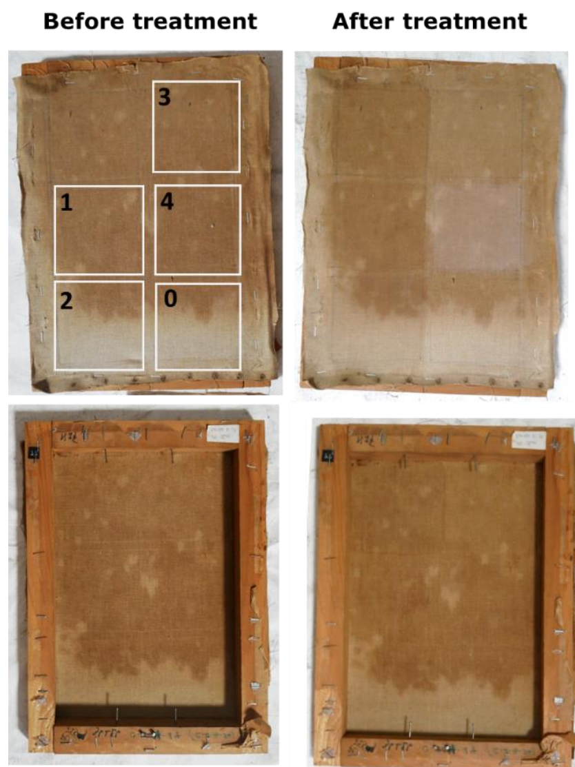
Figure 7.7: Lining canvas (high density n°1) before (0) and after treatment with MC+CNC (w) (1), MC+CNC+CaCO 3 (w) (2), MC+CNC (h) (3) and MC+CNC+MgO (h) (4).
