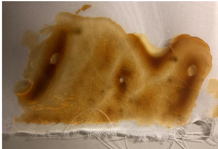
Figure B.10: Animal glue film after ageing. Note that the film has strongly degraded as seen by the strong darkening of the film, cracks have appeared and because the film had started to melt, it was put on the sailcloth seen on the picture.
