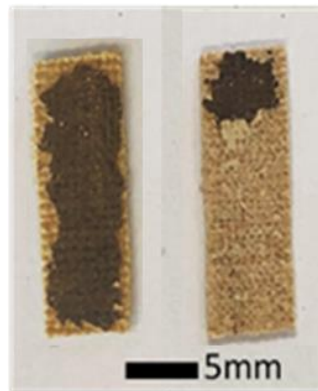
Figure 3.36: Picture of the same sample before (left) and after (right) removal of the priming layer. The sample was used as such for DMA-RH measurements.
