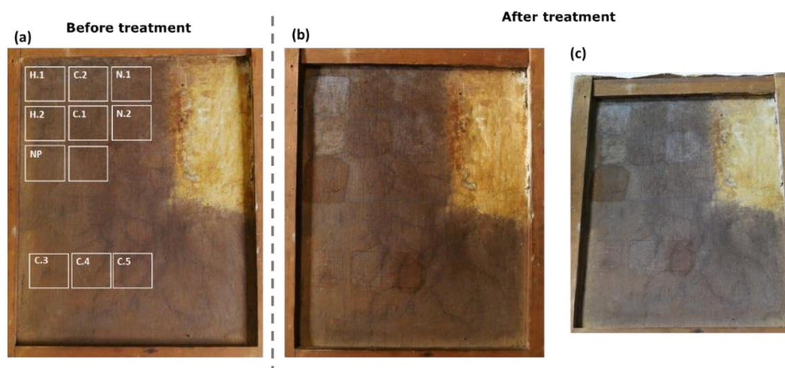
Figure 7.9: The musician painting before (a) and after treatment (b,c) with aqueous composite treatments MC+CNC (w) (C.1) and MC+CNC+CaCO 3 (C.2), the heptane-based composite treatments MC+CNC (h) (C.3), MC+CNC+MgO (h) (C.4) and the deacidification MgO solution in heptane (C.5), the nanocellulose dispersions CNF (NC.1) and CCFNF (NC.2) and the hybrid treatments Sil/PEI (H.1), Sil/PEI/CMC (H.2) and the solution of CaCO 3 nanoparticles (NP). The modification of the reflective index of the canvas after the application of the treatments is revealed by illumination of the canvas under raking light (c).
