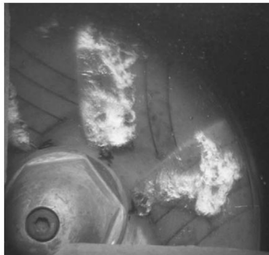
Figure 1.5: Attached cavity at the leading edge of a centrifugal pump [3].
