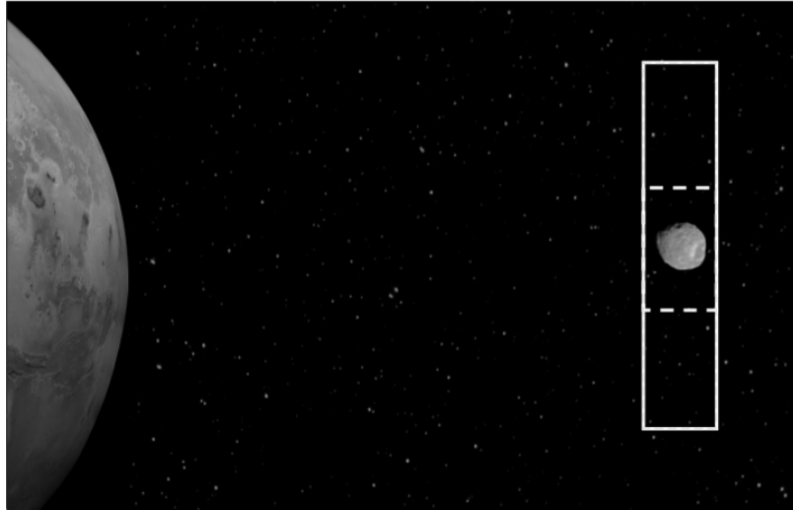
Figure 4.11: Potential use of background slit to view moons and mitigate for stray light from the host planet (not to scale). Original images credit: NASA.
