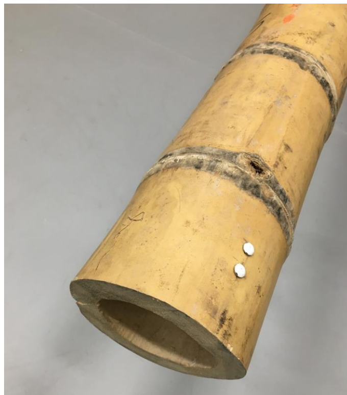
Figure 2. End section of bamboo pole and scanning reference markers
