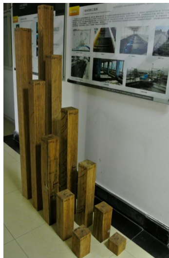
72 73 Fig. 1. PBSL columns with various length
