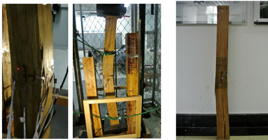
123 (a) Large lateral deflection
