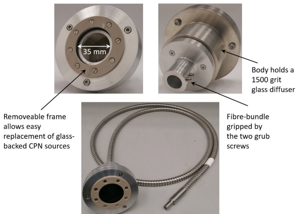
Figure 6-6: A practical LGUS source. The source element secured in the aluminium body shown in the bottom image is a PDMS-based CPN with 2.0 wt. % MWCNT and film thickness is approximately 20 \mu\text{m} .
