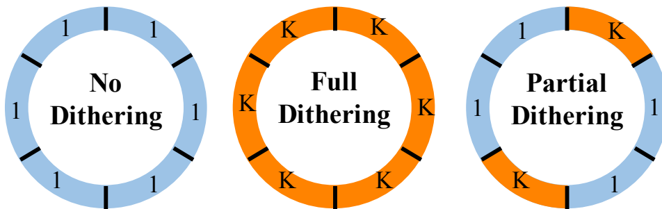
Figure 2. A comparison between no-dithering, full-dithering and partial-dithering when V = 6 and D = 3 . Each arc represents a tomographic view angle. The numbers on the arcs denote the number of exposures taken at the view angle. The orange arc means K -step dithering is implemented at the view angle, while a blue arc means there is only 1 exposure taken.
