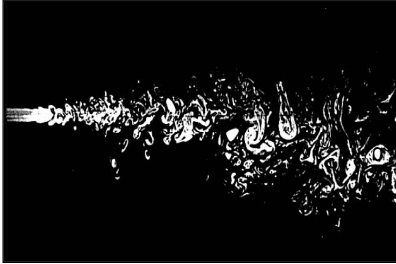
Figure 3.1: Photograph of a water jet, showing the transition from laminar to turbulent flow. The non-uniform, irregular structure of the flow is evident and appears as vortices of different sizes Figure from Frisch [1995], adapted from van Dyke [1982].
